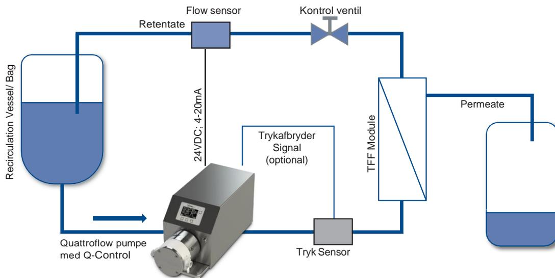
Quattroflow-anbefalet Flow Sensor: em-tec BioProTT™ FlowTrack plus eller FlowMCP with Clamp-On Transducer
