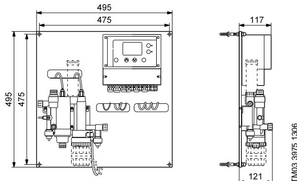
**Fig. 12** Dimensions, Conex® DIA-1-A, D1 (D2 / D3), Conex® DIA-2-A, D1 (D2 / D3), Conex® DIA-2Q-A, D1 (D2 / D3) preassembled systems for  $\text{Cl}_2$ ,  $\text{ClO}_2$ ,  $\text{O}_3$ , pH or redox (ORP)
