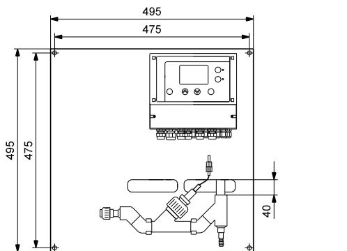
**Fig. 15** Dimensions, Conex® DIA-1-A, F, preassembled systems for fluoride
