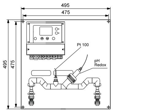
**Fig. 14** Dimensions. Conex® DIA-1(2 / 2Q)-A, P/R, preassembled systems for pH or redox (ORP)
