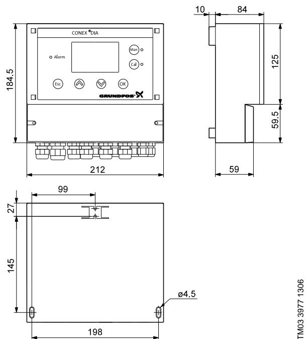
Fig. 9 Dimensions, Conex® DIA for wall-mounting
