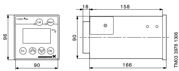
Fig. 10 Dimensions, Conex® DIA for installation in control panel
