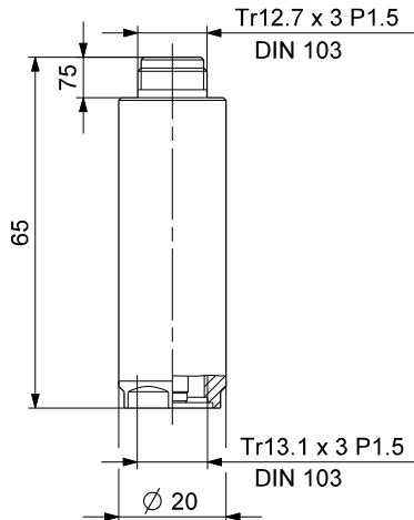
Fig. 17 Dimensions, impedance converter
